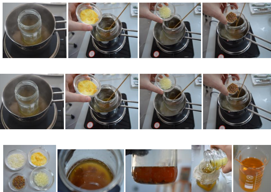
Fig. 3 – Details from the reconstruction of varnish recipes and details with four resins: dammar, mastic, amber and colophony
