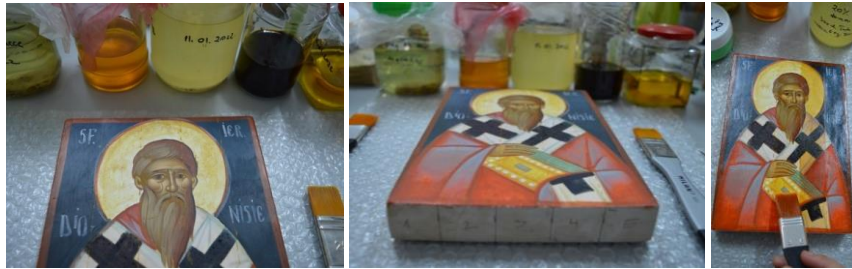
Fig. 5 – The new painted icon was divided into five strips and varnished with the reconstructed recipes
