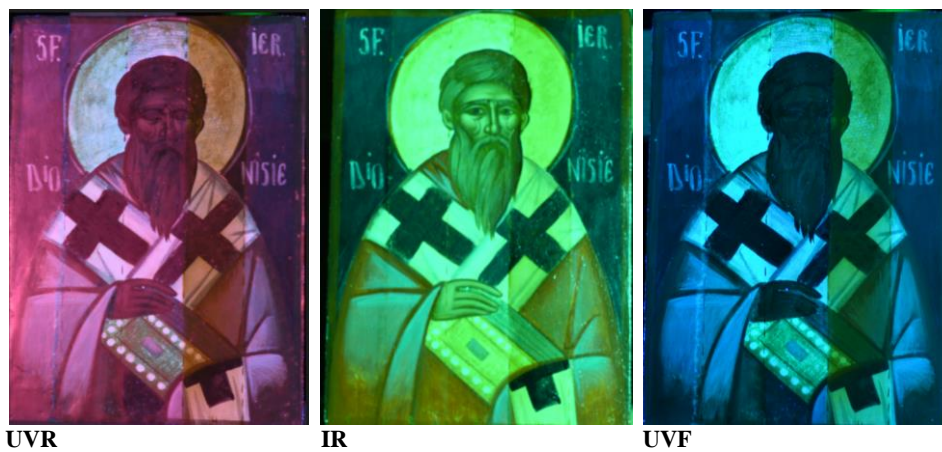
Fig. 8 – Reflected Ultraviolet (UVR), Infrared (IR) and Ultraviolet Fluorescence (UVF) photography of the icon showing the various vertical stripes brushed with the 5 (five) reconstructed varnishes
