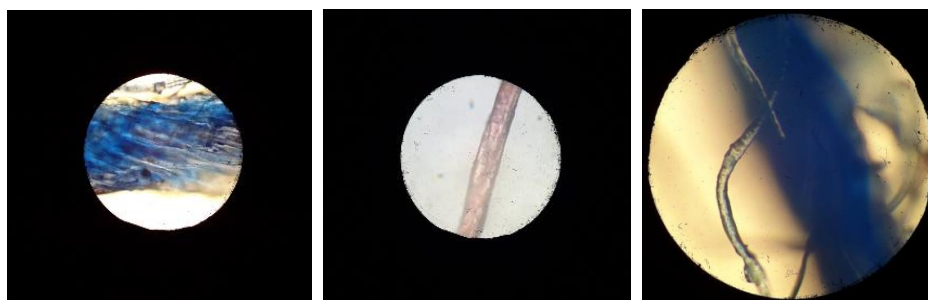
Fig. 6 – Detalii fire textile - bumbac (1000x, 40x)
